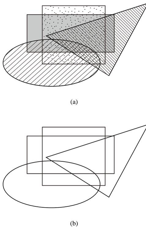
Figure 3 Intersection of four polygons. (a) Original polygons, (b) polygons generated by intersection.
