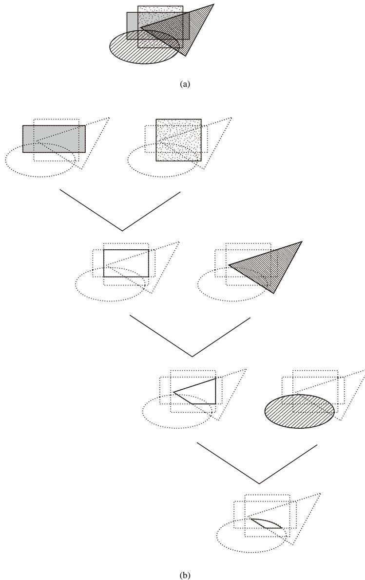
Figure 5 Construction of intersection tree from four polygons. (a) Original polygons, (b) tree construction process. The rectangles are chosen first to be replaced by their intersection. The triangle and ellipse are chosen in turn to generate a small polygon at the bottom of the tree. Dotted lines indicate the location of original polygons.
