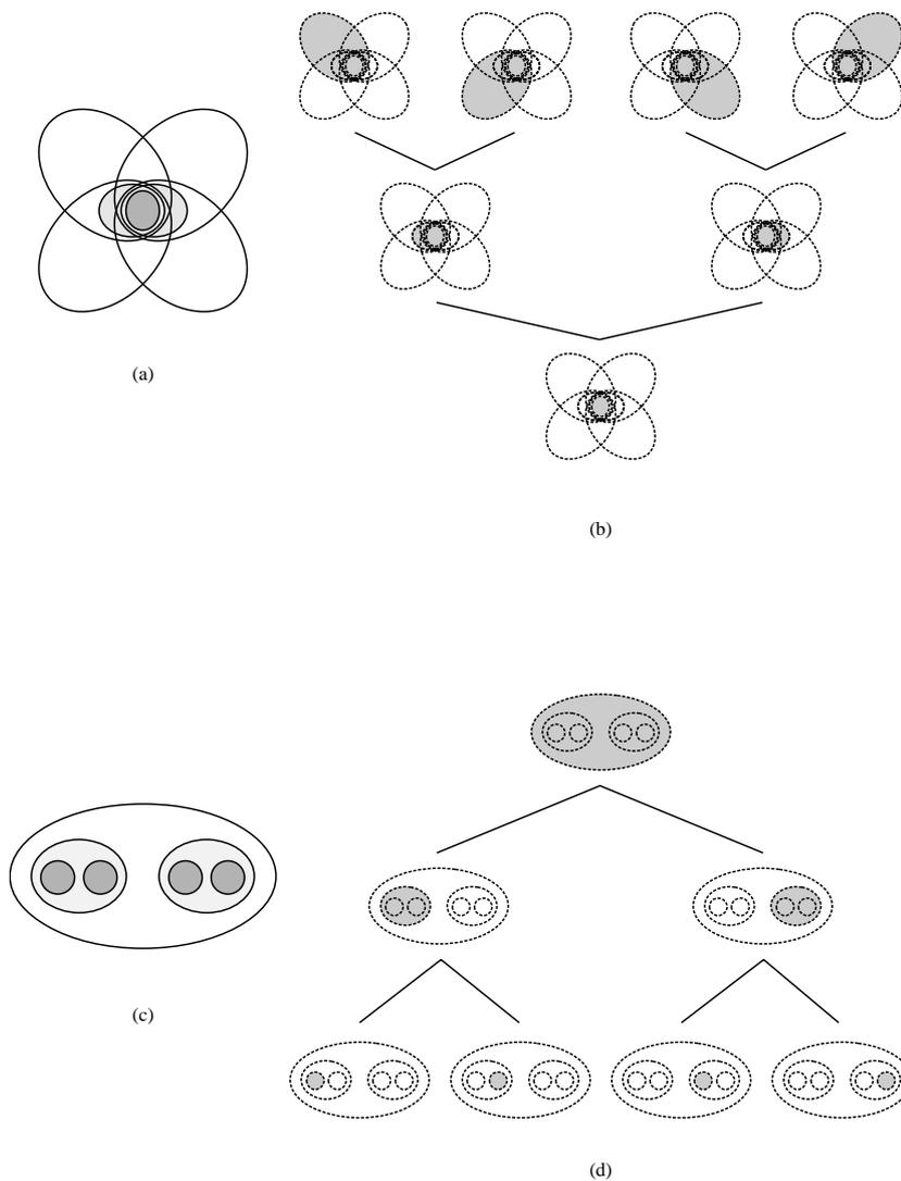
Figure 6 Hierarchical structures and their graph representations implicitly assumed in intersection and union trees. Hierarchical structures of three level polygons assumed in (a)(b) intersection tree, (c)(d) union tree.
