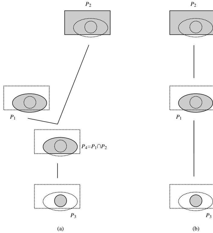
Figure 9 Link simplification. (a) Three polygons  $P_1$ ,  $P_2$ , and  $P_3$ , where  $P_1$  and  $P_2$  are almost hierarchical. (b) Direct connection of  $P_1$  and  $P_2$  by a single link.
