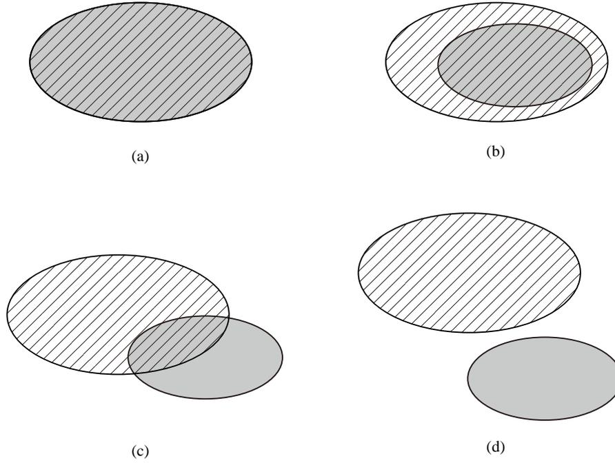
Figure 1 Relations between a pair of polygons. (a) Equal, (b) hierarchical, (c) overlapped, and (d) disjointed. These four relations are mutually exclusive.
